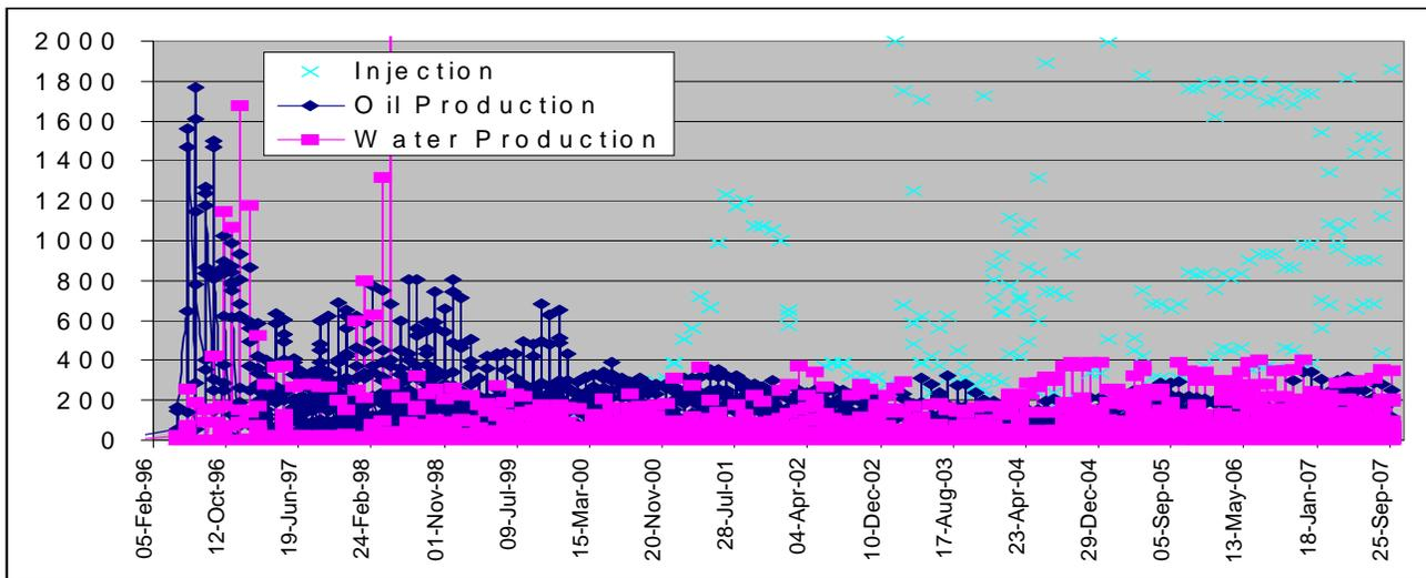
**Fig. 10 Production history of Moldabek field. It is well seen in this figure that these fields are producing mainly water and are depleted to great extent since 2000. This fact is perfectly matching the pattern of hydrocarbon spatial distribution as revealed by IPDS survey (Figures 8 and 9). The last shows that the studied fields are mainly presented in blue color reflecting prevailing water cut production rather than oil. Oil and water production data are expressed in tons.**
