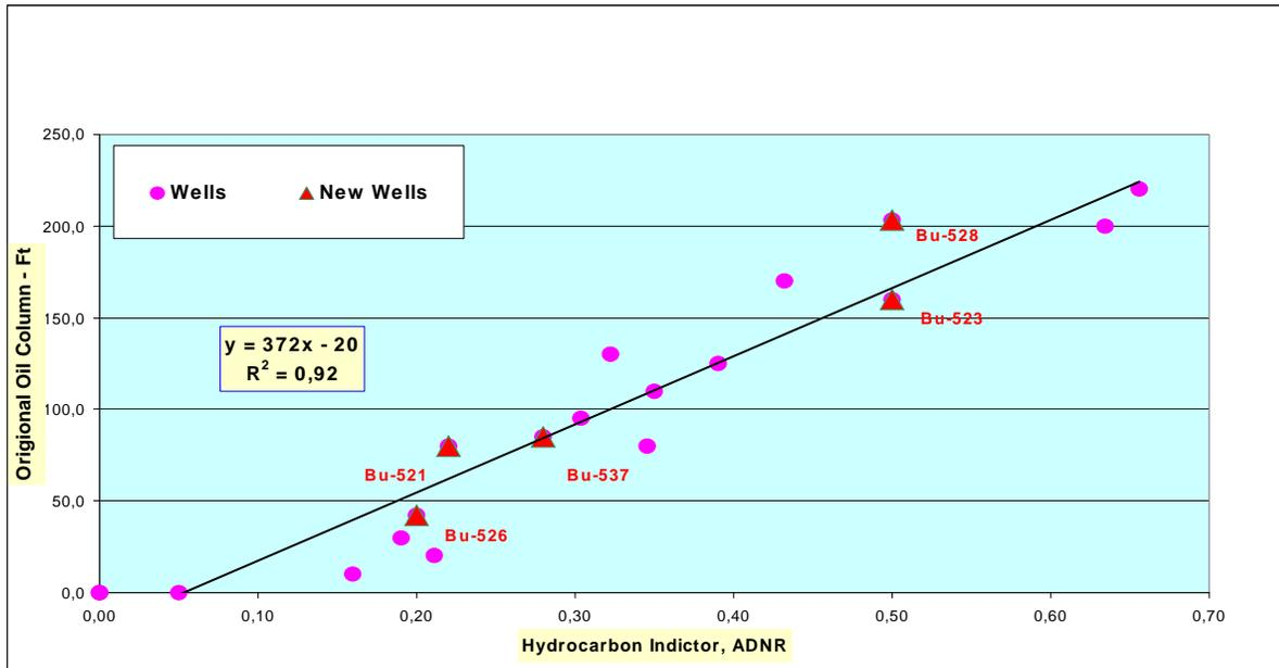
**Figure 3 Correlation between the IPDS hydrocarbon indicator and net oil pay zone thickness in the UAE field B. Correlation coefficient is in the order of 90%**
