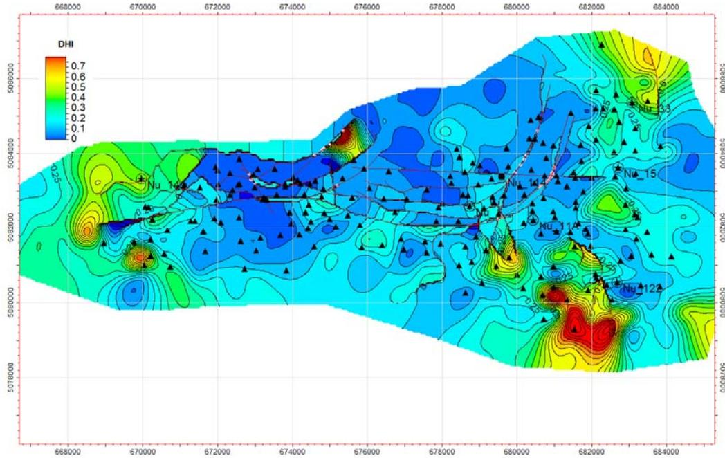
**Fig. 9 Map of spatial distribution of hydrocarbon accumulation in the Nurzhanova Field. Color scale represents direct hydrocarbon indicator, as function of cumulative net oil pay zone thickness.**
