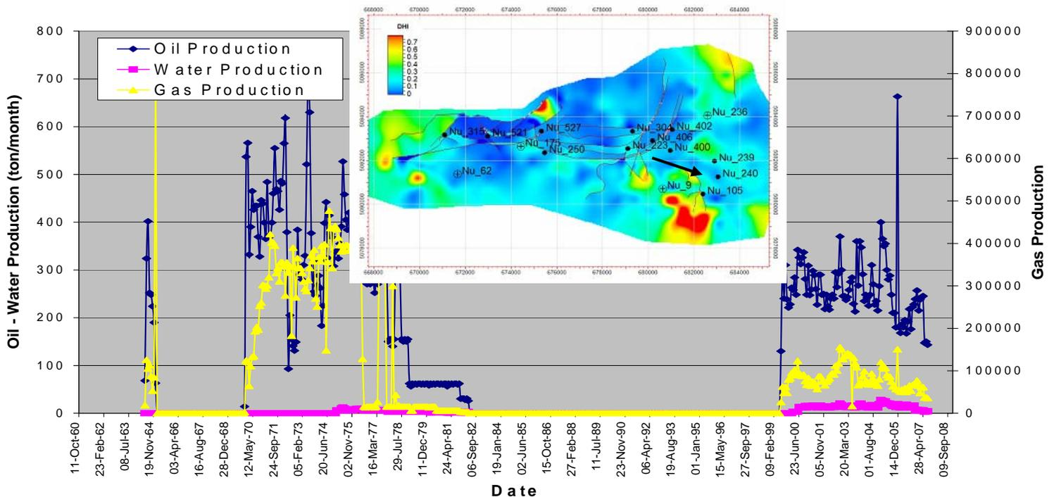
**Fig. 11 Correlation of production data and IPDS survey results for well CVP\_105:J3\_II-CE-1. Oil production data are expressed in tons; gas production data are expressed in M<sup>3</sup>**
