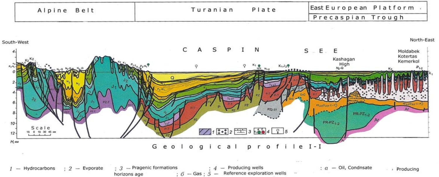
**Fig. 6** Regional geological profile in the Pre-Caspian basin where the right part of the figure is presenting the North Caspian basin, related to the East European platform. Here, an IPDS survey for HC exploration and reservoir monitoring was carried out in Moldabek, Kutertas and Nurzhanova fields in 2006-2007
