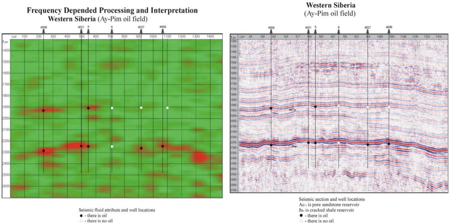
**Fig. 4 Passive low-frequency seismic profile showing detected oil accumulation and their correlation to well production data (Goloshubin et al., 2006)**
