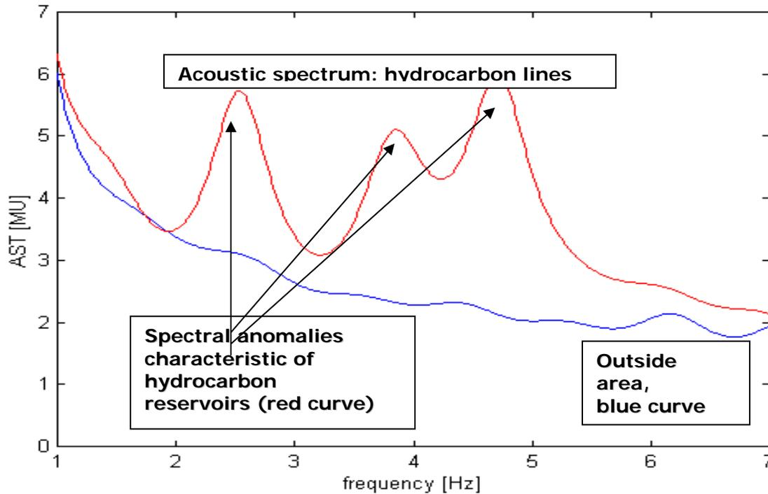
Fig. 1 Comparison of spectra and signals recorded during the IPDS survey. Live Data: Spectral analysis of signals recorded in the northern part of the UAE-Q field
